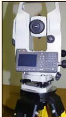
This Sokkia Total Station device is dedicated solely to measuring a scene.
